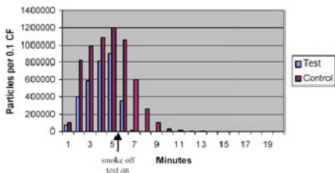
The differences in the initial air densities were much greater for the 1 µm than for the 0.3 µm particles. After 5 min of operation, the particle density with the unactivated filter in place was about 25.3 percent lower than without the filter in place.
