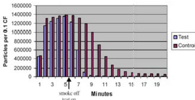
During this initial 5-min period, the test experiment shows the particle densities with the filter in place but without electronic activation.
